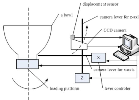
Fig 1. Schematic of system structure
