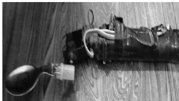
Fig.7. Hardware model of the Self-stabilizing Spoon for Parkinson person
