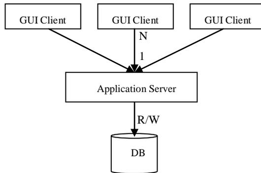
Fig 1. C/S two-tier architecture
