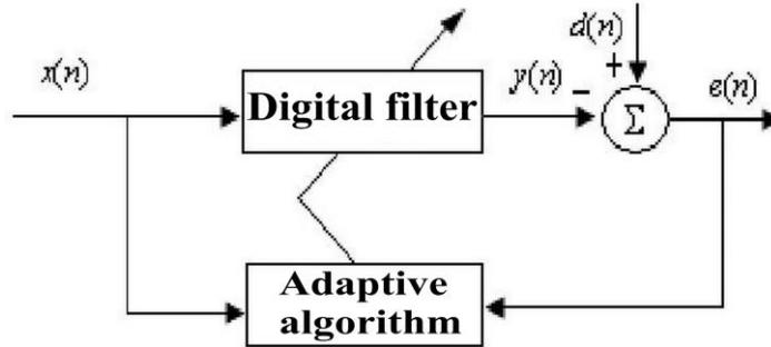
Fig. 5. Schematic diagram of adaptive filter algorithm
