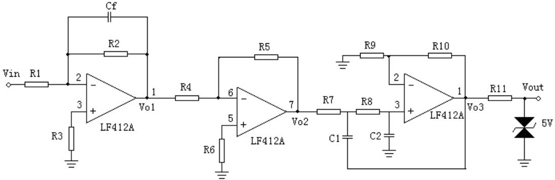
Fig. 2. Signal Conditioning Circuit
