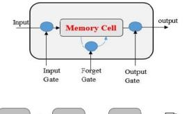
Fig.1. LSTM cell [15].
