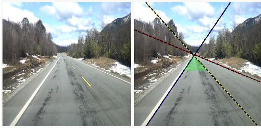
Fig.7. Detection of the center line based on the vanishing point.
