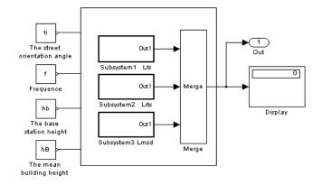
Fig 2. Modeling the COST231-WI model
