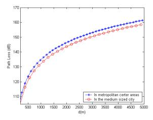
Fig 8. Path loss in different environment
