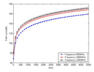
Fig 7. Path loss for different frequencies
