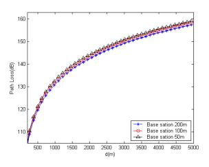
Fig 6. Path loss for different base station height
