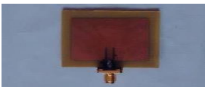
Fig.5.Fabricated inset fed short edge patch antenna with ground plane dimensions 6h+L and 6h+w
