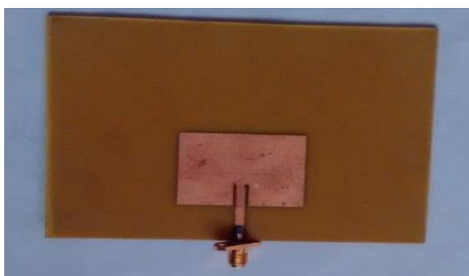
Fig.11.Fabricated inset fed patch antenna with triple ground plane.
