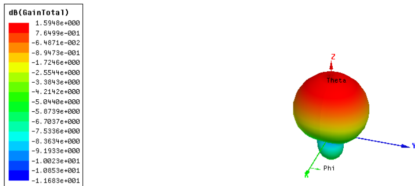
Fig.8.Gain plot of the inset fed short edge patch antenna with ground plane dimensions 6h+L and 6h+W
