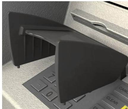
Fig.6. Example of a shell that hides the user's finger when spinning the color when on the ATM screen
