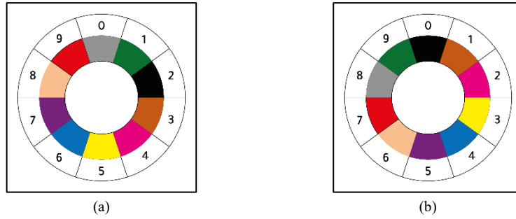
Fig.3. Color wheel: (a) after spinning with a random degree in the middle of the first CWPIN session, (b) just after entering the tow last PIN digits
