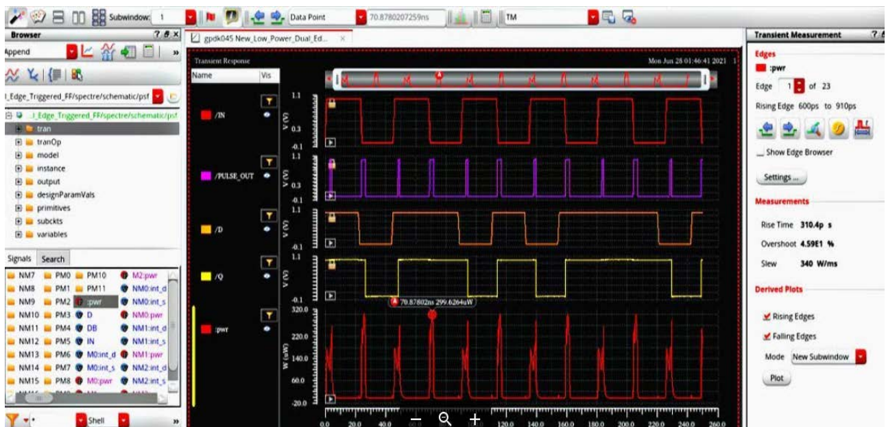
Fig.20. Analog simulation with spectre of New Proposed low power DETFF
