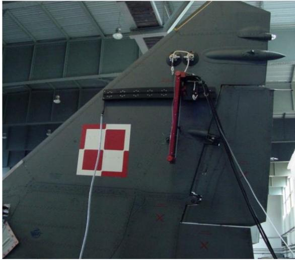
Fig. 1. MiG-29 composite vertical stabilizer during NDT inspection.
