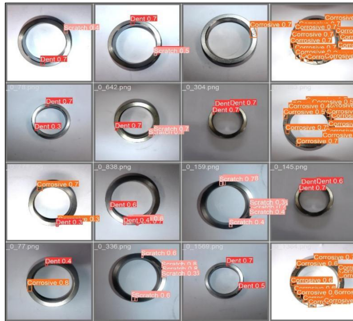
Fig.14. Defect detection and classification by YOLO v8 model
