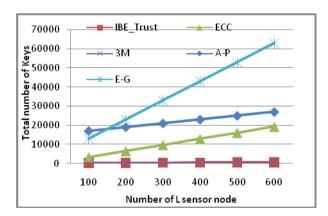
Fig.2: Pre-Loaded Keys in Networks
